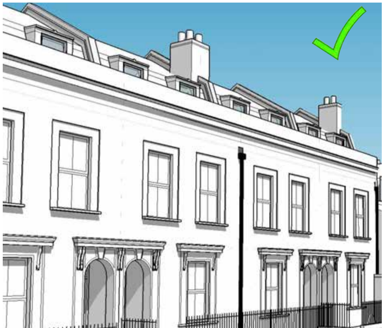
Mansard with larger set-back behind parapet wall
